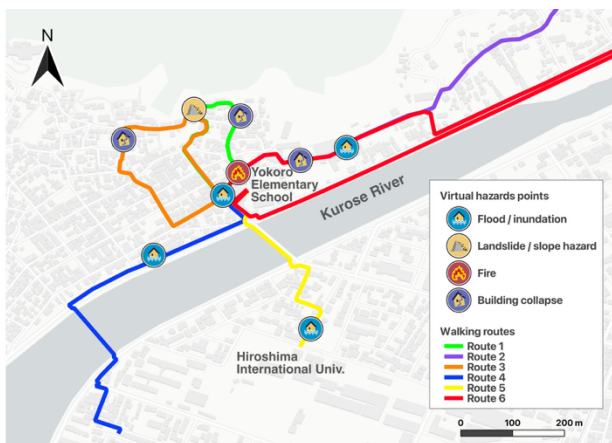
Figure 6. Field-deployment map of the Hiro area case in Kure City, showing the walking routes, AR hazard points, and surrounding base-map context used for disaster risk interpretation. The map illustrates how public GIS resources, local field inspection, and route-based scenario design were integrated into the MUSUBOU-AR deployment workflow.
