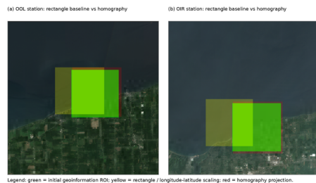
Figure 4. ROI localization comparison. Green is the reference ROI, yellow is rectangle scaling, and red is homography projection.
