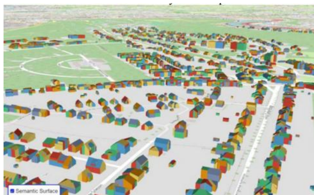
Figure 7. Class-based rendering applied to a building material characterization scenario on the Sart-Tilman dataset, using randomly assigned class attributes on all semantic surfaces.
