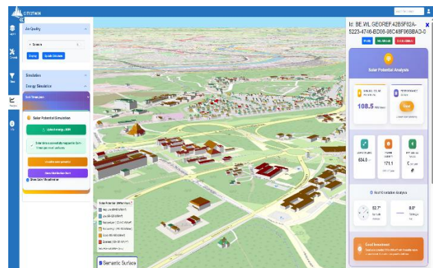
Figure 5. Surface-level photovoltaic potential visualization of the Sart-Tilman district in City2Twin: individual roof surfaces colored by performance class and per-surface assessment panel: annual yield, performance class, area, power density, orientation, and automated installation recommendation for a selected roof surface.
