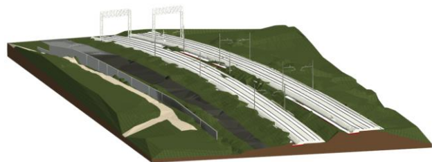
Figure 6. Federated BIM model of the railway section, consisting of the terrain model made in Revit® and the tracks modeled in Civil 3D® and exported in IFC 4.3 format, integrated in a single coordinated environment.
