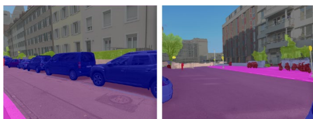
Figure 3. Examples of the resulting semantic segmentation outputs for street-level images visualised using the Cityscapes colour palette, where each colour represents a different class.
