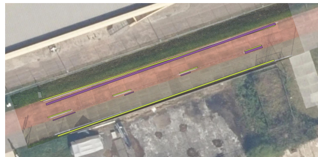
Figure 4. Extracted road-marking corner points (purple: S1; green: S2) overlaid on drone imagery of the case-study area.
