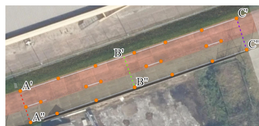
Figure 2. GNSS points for the local-to-global datum transformation, pictured on drone shots taken during the case study, including the cross-profile lines of Figure 6 and 7.
