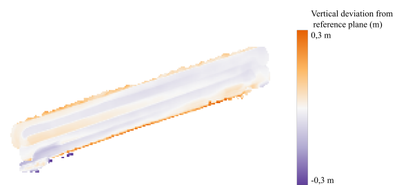
(b) Vertical variation of S2 between the point cloud and the fictitious linear plane.
