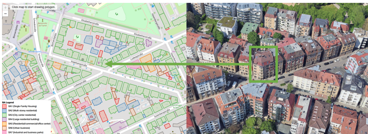
Figure 4. City center (BA3) assignment of a building with Google Earth comparison
