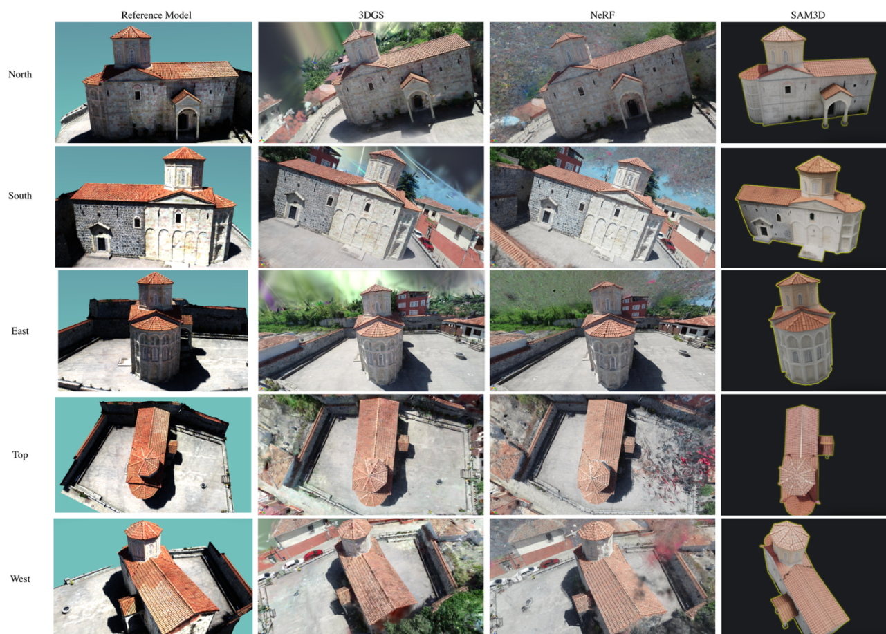
Figure 2. Visual samples from experiments and the photogrammetric reference model.
