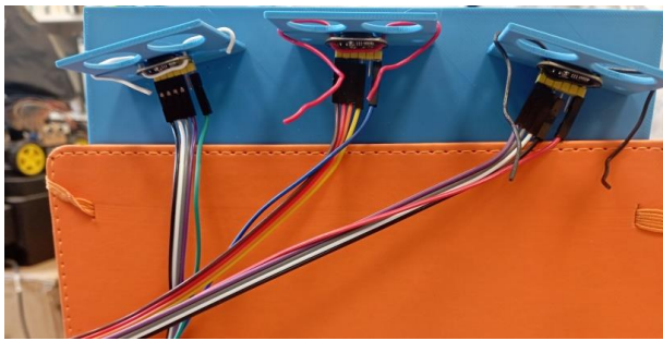
Figure 4. 3D printed sensor holder with TOF400C-400cm laser distance measurement unit
