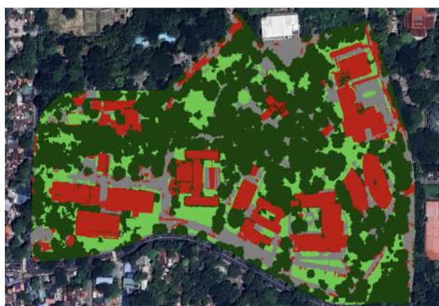
Figure 6. Resulting surface classes: Trees (green), Vegetation (light green), Buildings (red) and Pavement (grey).
