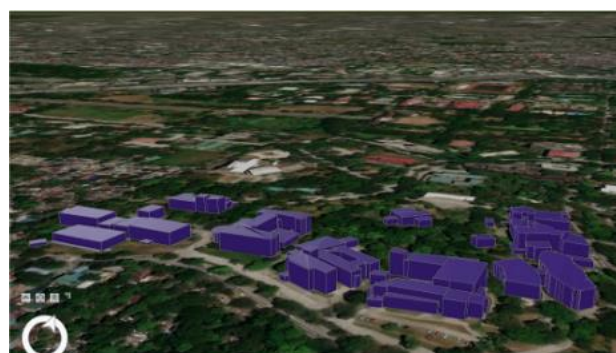
Figure 5. LOD 1 3D model of the Engineering Complex.
