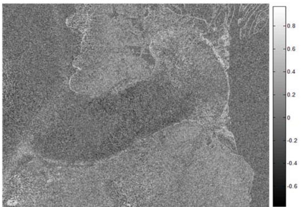
Fig.5. Coherence map of one part of the outlet area of the Taku Glacier generated from two TerraSAR-X repeat cycle scenes with 11 days interval.
