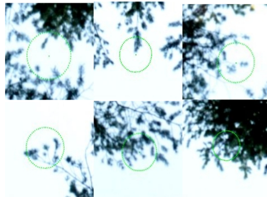
Figure 7. Examples of LMS-Q680i ( 1/e^2 ) first-echo footprints in pine crowns, showing an intensity gradient with DN values of 10, 15, 26, 37, 46, and 89. The largest value is associated to a single echo, while the rest are of type first-of-many.
