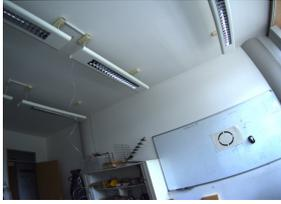
**Figure 7:** Sample image of our vignetting measurement series. The measurement target is the area inside the black circle on the A3 sheet mounted on the white-board.
