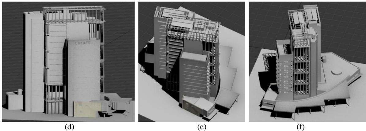
Figure 7: Example of complex CREATE building, (a) an image from UAV; (b) sample point cloud from Mobile Mapping system; (c) terrestrial image sample collected by NIKON D7000; (d)(e)(f) views onto the 3D model of the CREATE building, produced by integrating the data from UAV, point cloud and terrestrial images.
