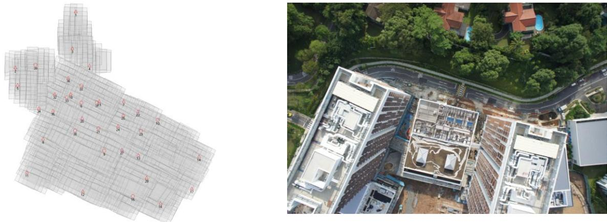
algorithm and a following exhaustive search strategy to deal with failure matching. The result of bundle adjustment using APERO is shown in Table 1. The RMSEs computed from 11 check points give 7 cm planimetric and 6.5 cm height accuracy. These values, slightly above the one-pixel mark (5 cm) are acceptable considering the fact that we are dealing here with natural control and check points.
