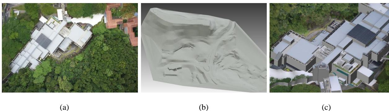
Figure 5: Results of NUS campus modeling: (a) one of the UAV images; (b) measured terrain; (c) zoom-in result of a textured building model.
