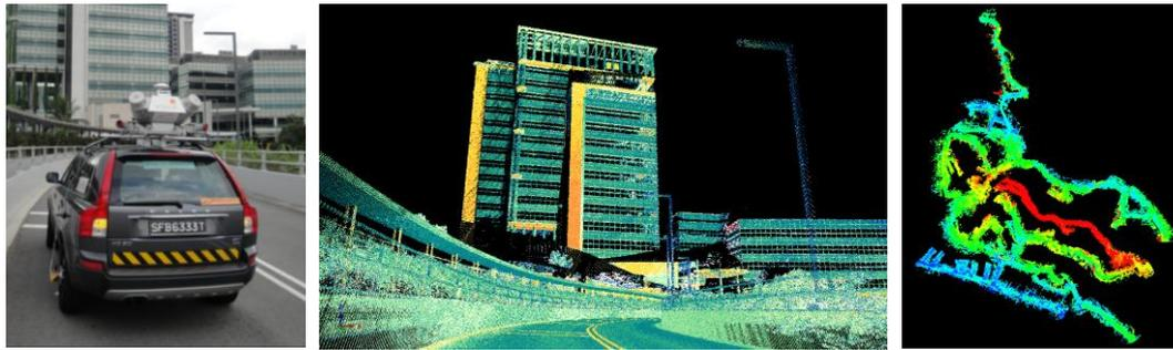
Figure 3: Mobile Mapping System (left), example point cloud data at CREATE buildings (middle) and MMS campus trajectory.
