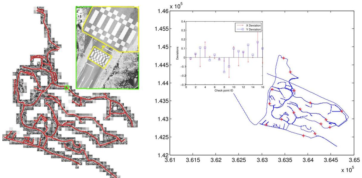
Figure 4: Left: Overview of NUS campus point cloud intensity data. Right: Distribution of check points and their coordinate differences at X and Y directions (Unit: meter).
