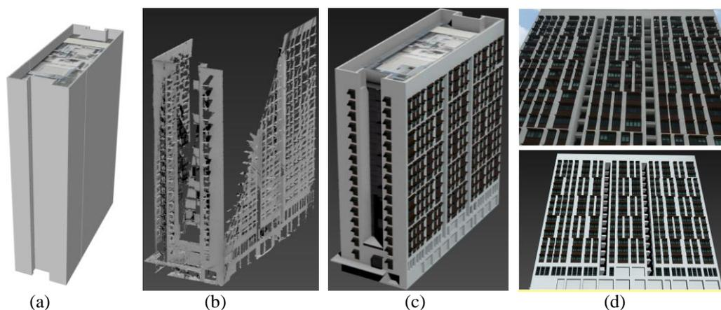
Figure 6: Example of a complete building model, (a) roof model from UAV images, (b) wrapped mesh from MMS point clouds, (c) complete model by integrating roofs and façades, (d) façade image (up) and 3D model (down).
