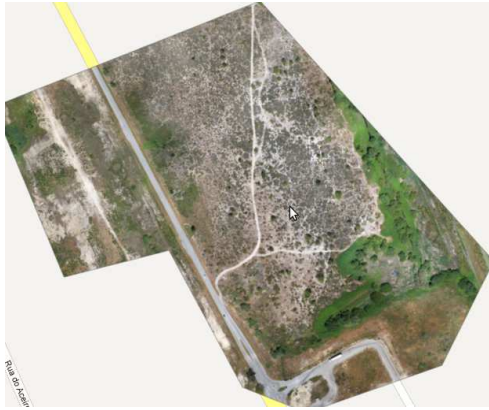
Figure 2: Example of an orthomosaic obtained from a set of aerial photographs with an average resolution of 6.9cm, obtained using the Spin.Works S-20 system.
