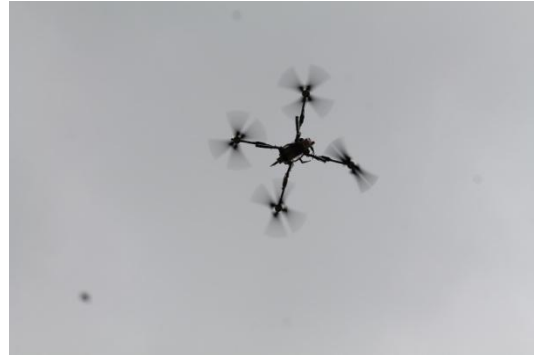
Figure 4.600 mm carbon rod coaxial quad
