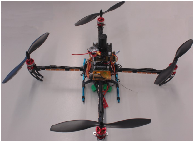
Figure 5. B110 receiver mounted to a Quadcopter-platform
