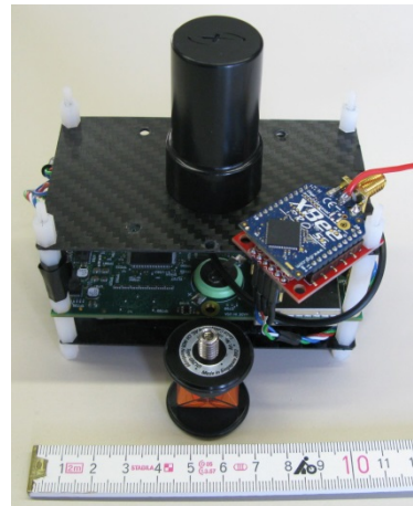
Figure 3. TOPCON dual frequency receiver OEM1 with Xbee radio module and dual frequency antenna Moxena M1227HCT-A-SMA (optional: 360°miniprism for target tracking with a tachymeter)
