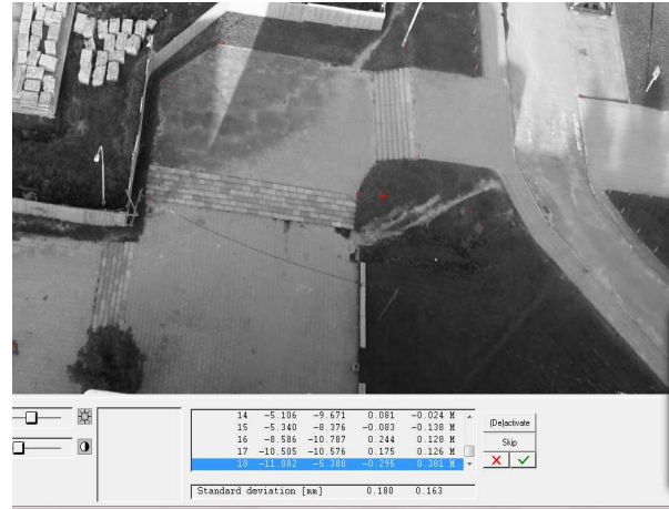
Figure 5. Fragment of results from exterior image orientation – UAV Photogrammetry
