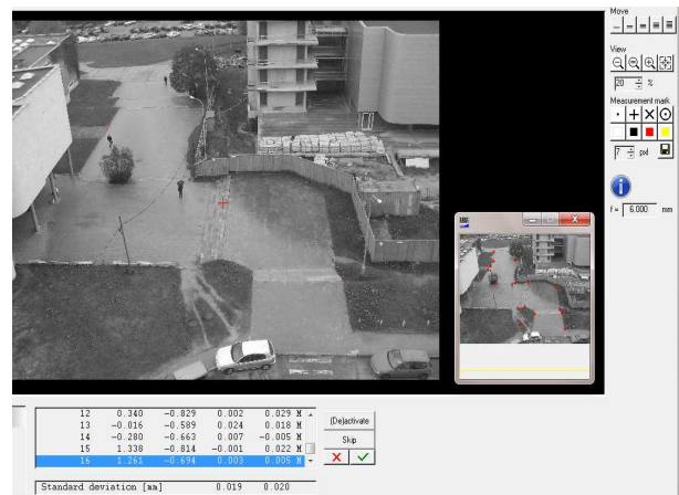
Figure 6. Fragment of results from exterior image orientation – Close Range Photogrammetry
