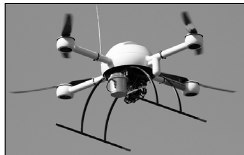
Figure 1. UAV md4-1000 with RSD and photo camera as a payload
