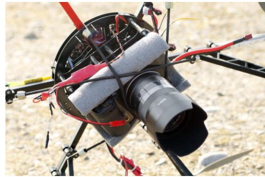
Figure 3: Sony RX1 in hexacopter pod with dampers.
