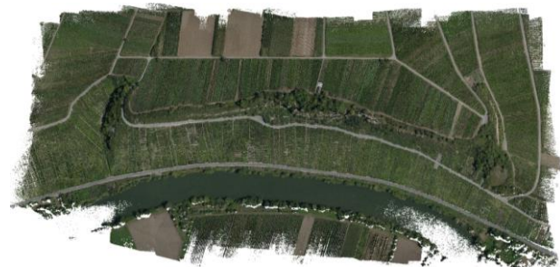
Figure 1: DSM from dense matching.
