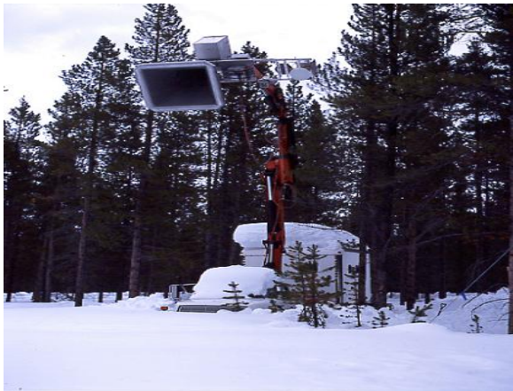
Figure 1 . L and Ku band radar at Fraser (Saint-Martin et al, 2003)
