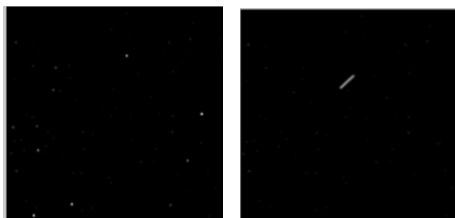
Figure 12. The detected stars (left) and the remained satellite streak (right)
