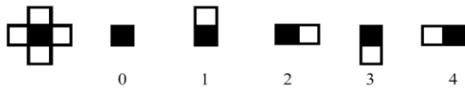
Figure 3. First-order neighbourhood system and its division into cliques. The black squares represent the site of interest and the white squares represent the neighbouring sites.
