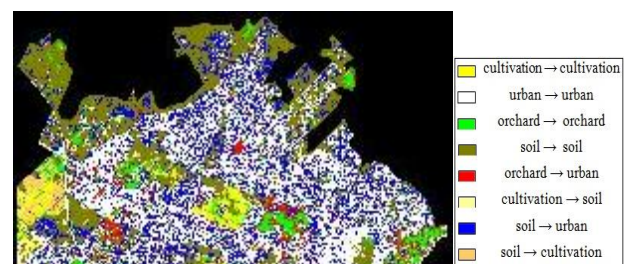
Figure 4. Output of defuzzification step of spectral-temporal combined analysis of Sugeno fuzzy integral operator
