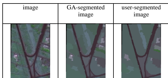
Figure 3. The result of image segmentation by using parameters optimized by GA and the user
