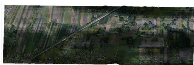
Figure 5. Point Cloud generated from low quality images (poor weather condition)
