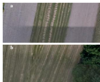
Figure 9. Example radiometric imperfections of automatic mosaicking process
