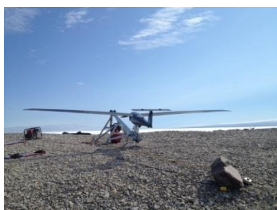
Figure 12 : Onshore pneumatic launch site
