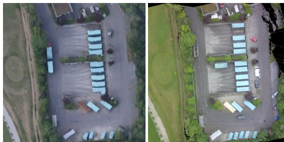
Figure 3. Comparison between 4K orthophoto (left) and MAV orthophoto (right) of the same area
