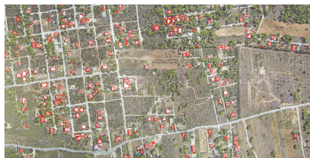
(c) The detected building footprints after the fusion process superimposed to the true orthomosaic
