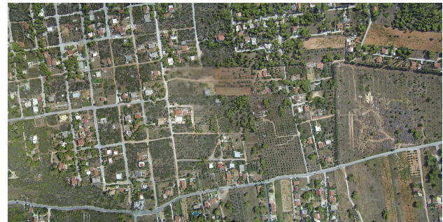
(a) The resulted orthophotomosaic (approximately 13.500 \times 7.000 pixels) with a spatial resolution of 8\text{cm} .
