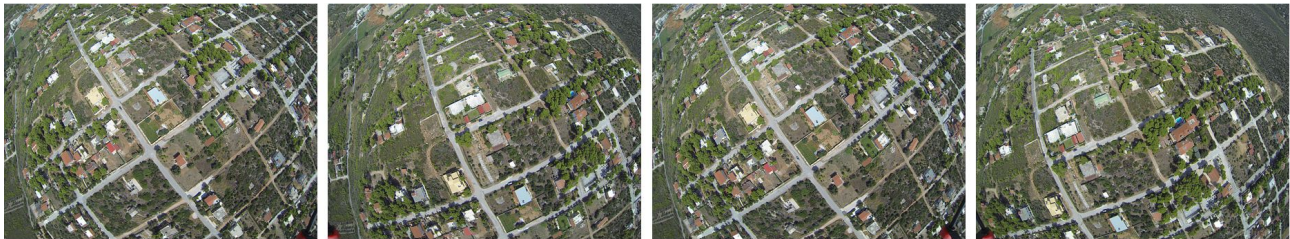
(b) Different views from the low-cost GoPro camera with important geometric distortions due to the fish-eye effect
