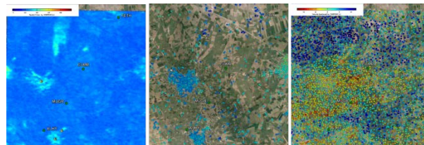
Figure 7. Average spatial coherence (left) and differences between processing approaches: PS InSAR (middle) and Quasi PS InSAR (right) over Cumra area from ERS data. Right image is considered as wrong result due to large number of noisy pixels as input for the processing
