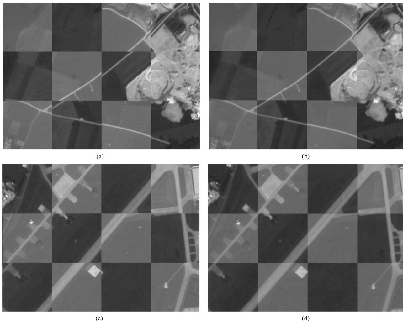
Figure 6: Chessboard overlays of overlap areas of the two QuickBird images. Figure (a) and (c) before, and (b) and (d) after the image transformation.
