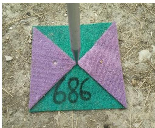
Figure 3. Artificial Ground Control Points Marker
