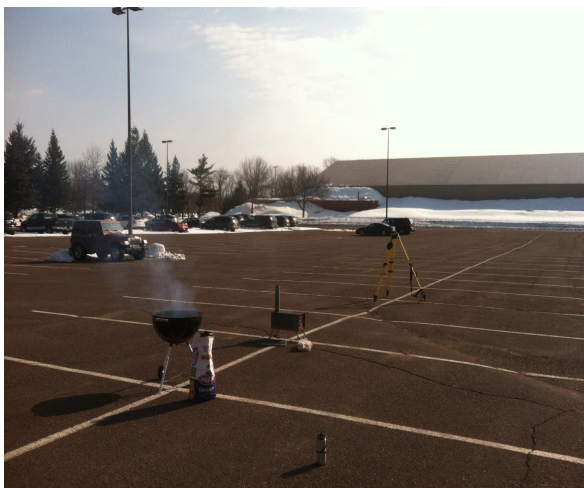
Figure 4. Experimental heat sources for testing UAV system.
