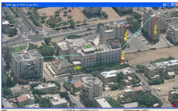
Figure 5. Height and distance measurements (Aeromap, 2006)
