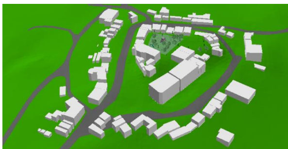
Figure 8. LOD1, "Block model" of old town and neighboring buildings, w/o roof structures
