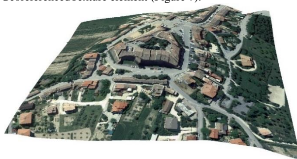
Figure 7. LOD0, 2.5D Digital Terrain Model over which an aerial orthophoto is draped.
