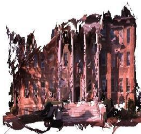
Fig.7- 3D reconstruction from Video only with the back pack system
