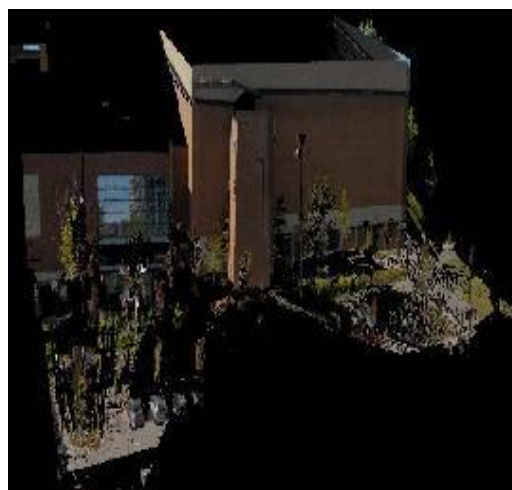
Fig.12. Textured point cloud model with laser and Images. (Source- Ming et al., 2009).
