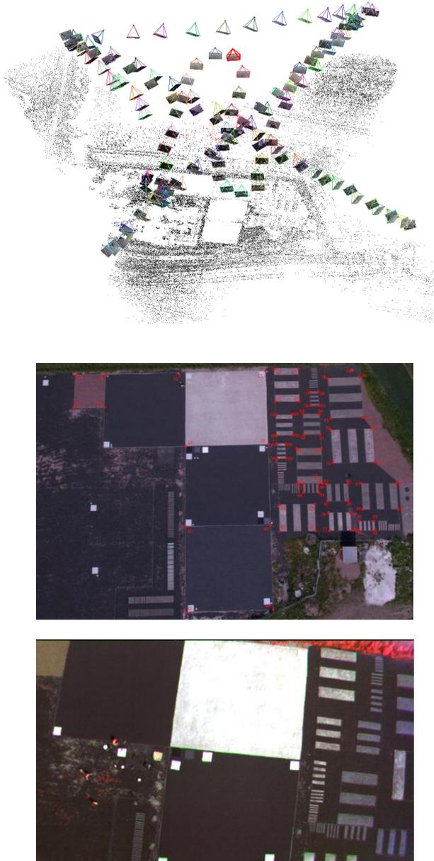
Figure 5. Traceable UAV campaign in Sjökölla remote sensing test field. From top: the image block with three vertical flight lines and two crossing oblique bi-directional flight lines; sample RGB image with ground control points; sample FPI image.
