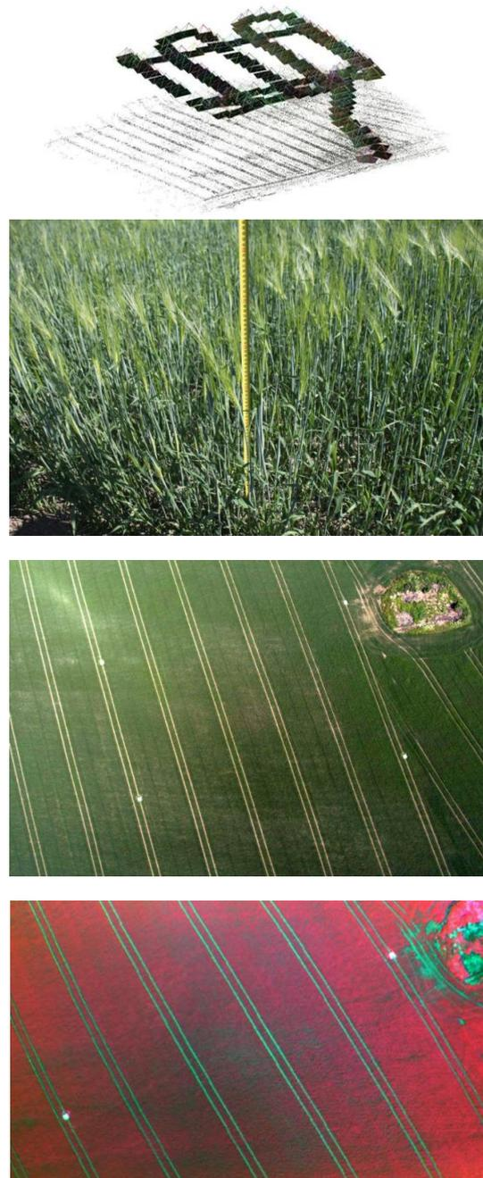
Figure 6. Traceable UAV campaign in Vihti agricultural test field. From top: the image block with five vertical flight lines and two crossing flight lines; ground view; sample RGB image; sample FPI image.
