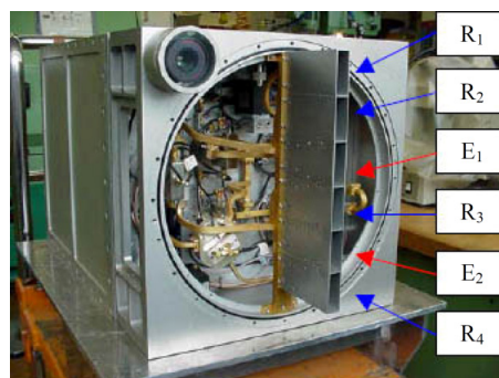
Figure 1. MEMPHIS Ka-band interferometric antenna. E1, E2: transmit horns, R1–R4: receive horns. Only one transmit horn can be used at a time.
