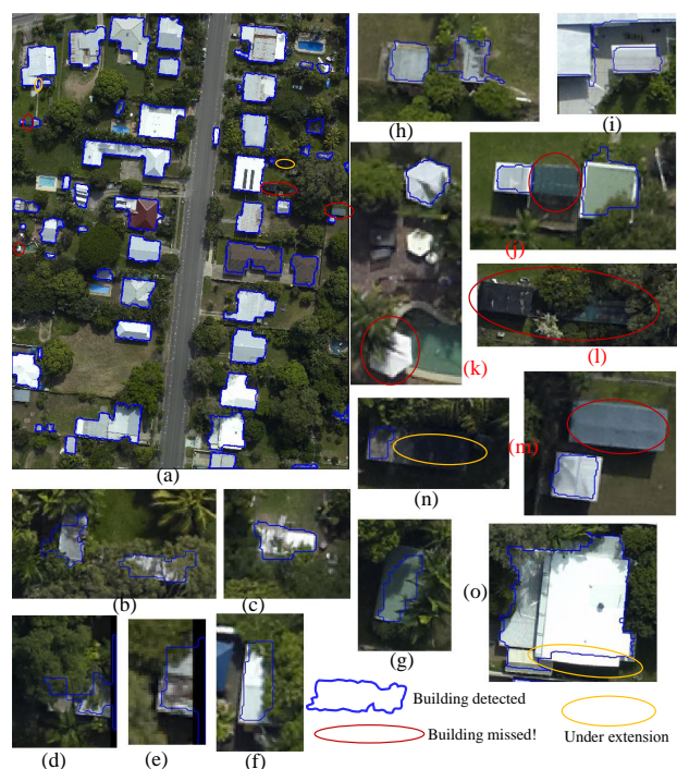
Figure 8. (a) Building detection on AV data set, (b)-(g) Magnified version of the buildings detected under complex scene, (h)-(i) Boundary over-extension, (j)-(m) Undetected buildings, (n)-(p) Boundary under-extension
