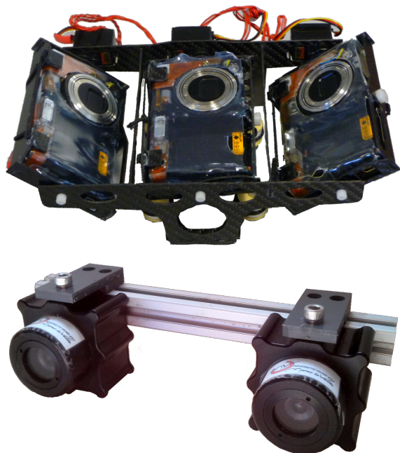
Figure 3: The developed payloads. Top: the tri-camera sensor, used on the Faucon Noir UAV. Bottom: the binocular stereoscopic rig, currently used on an underwater robot (sealed housings can be removed when the rig is used on a flying vehicle).
