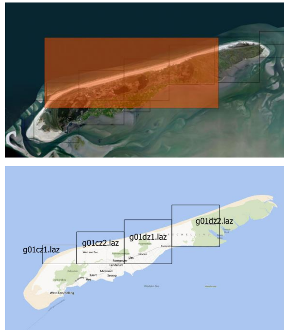
Figure 5: Example result of a spatial query visualized using QGIS. In the top image the red box represents the search polygon. The bottom image shows the tiles that are completely within the search polygon. The MongoDB spatial query delivered four tiles on the coast of the Netherlands.
