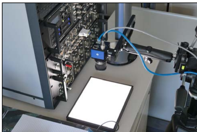
Figure 5: Custom-built „natural white LED“ flat field with frame imaging camera during daylight
