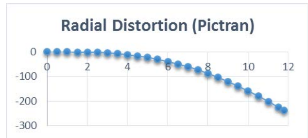
Figure 4: Radial Distortion [ \mu\text{m} ] as function of radius [mm] (APO Xenoplan). Software used: Technet Pictran
