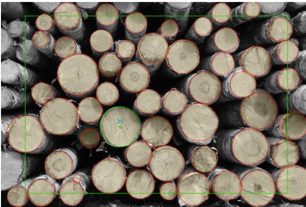
Figure 7. Result of work of accumulator for circle hypotheses
