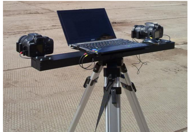
Figure 2. Portable photogrammetric system
