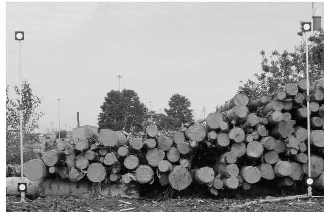
Figure 9. Log stack section with photogrammetric probes
