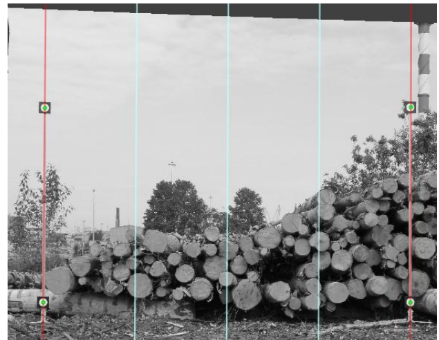
Figure 10. Log stack section orthophoto divided into sections for heights calculation
