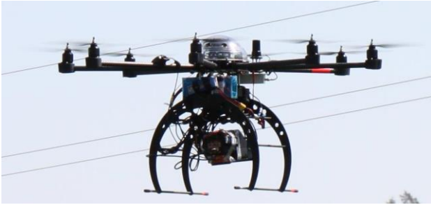
Figure 2. Mikrokopter UAV with the spectral camera.
