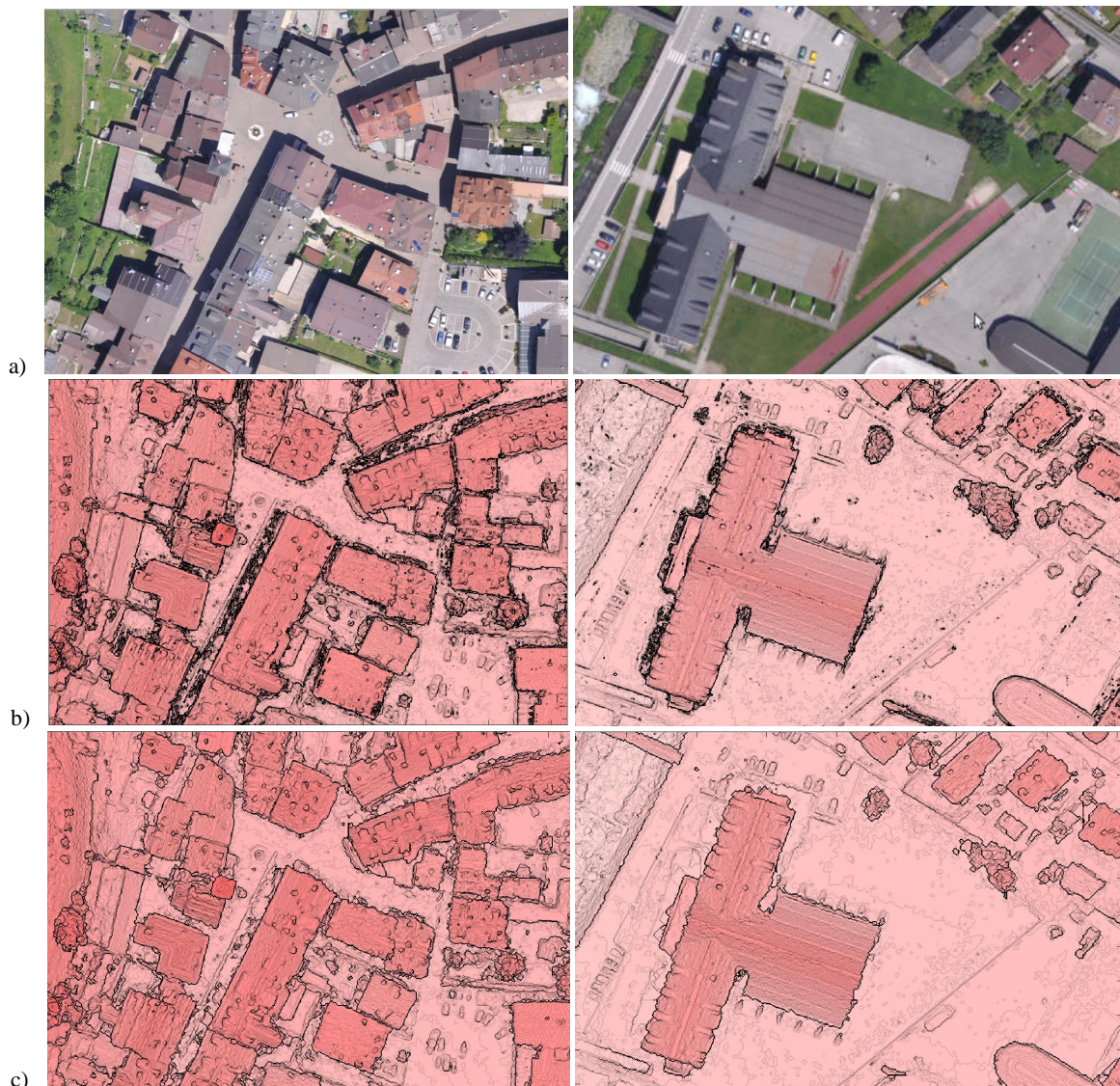
Figure 8: Qualitative comparison of real case: the true ortho-photo of the area (a), the DSM before (b) and after (c) denoising.
