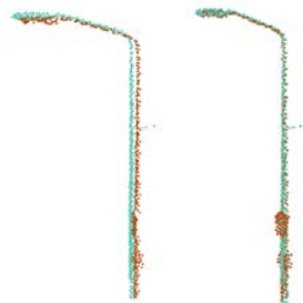
Figure 13 Two components on lamp posts overlaid using relative coordinates (left) and after ICP algorithm (right).
