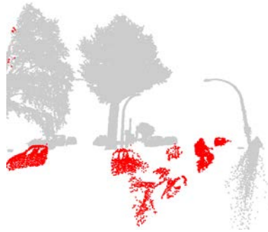
Figure 4 Dynamic objects (red) detected by using knowledge of a two sensor system.
