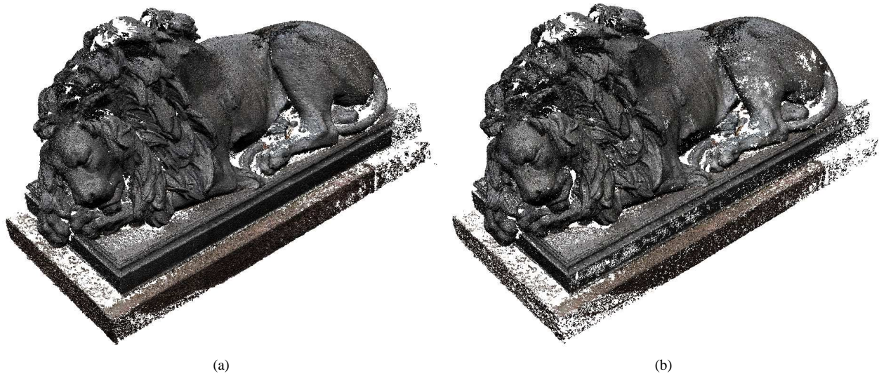
Figure 4: Resulting oriented points of the lion data set. (a): RQT error threshold \epsilon = 1.0 . (b): RQT error threshold \epsilon = 1.2
