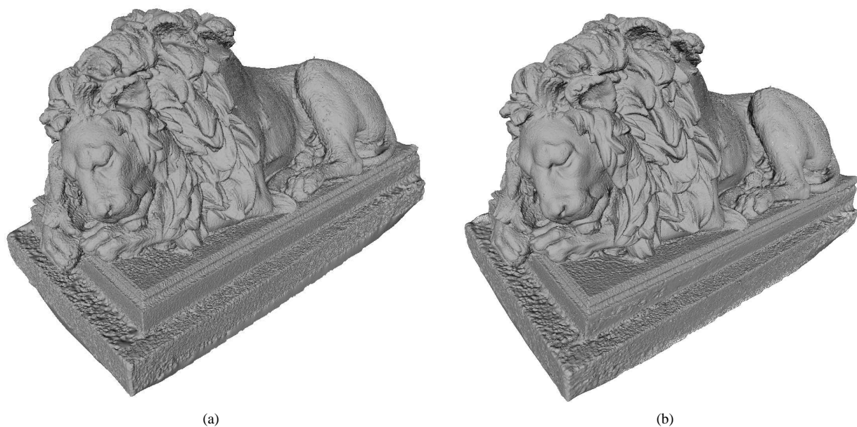
Figure 6: Poisson reconstructions based on our oriented point sets. (a): RQT error threshold \epsilon = 1.0 . (b): RQT error threshold \epsilon = 1.2
