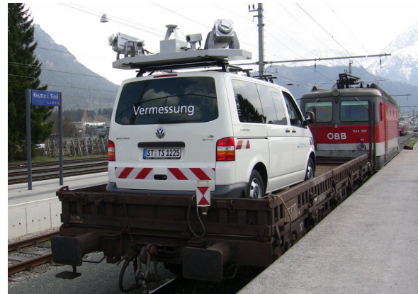
(a) The Optech Lynx Mobile Mapper on the back of a train wagon.
