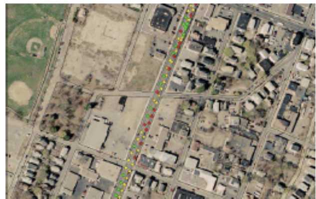
Figure 5. Automatically geo-located pothole clouds colored by severity (Angelini, 2006).
