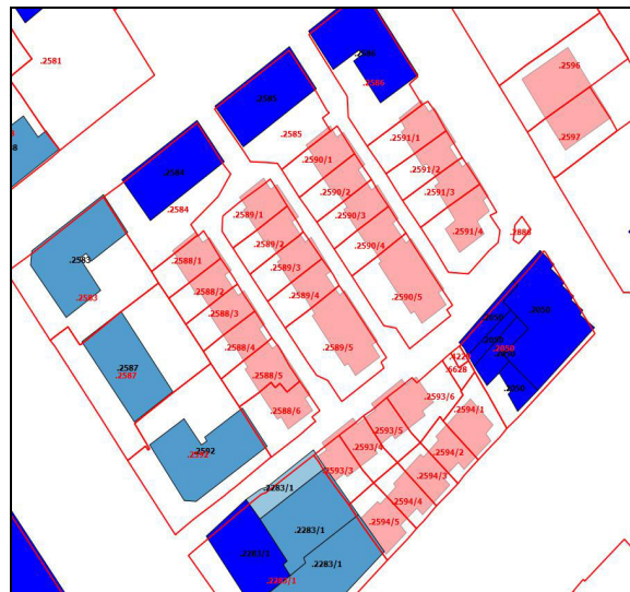
Figure 4 Example of overlay and intersection between land cadastre parcels (red lines, with IDs) and topographic map polygons. The pink polygons need to be split, as they cover multiple cadastre IDs. Cadastral IDs are assigned automatically to the polygons the other polygons, depending on the ratio of overlapping area.
